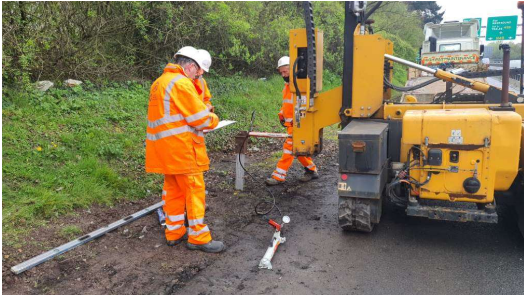
Testing of the crash barrier posts on the N40 westbound verge
