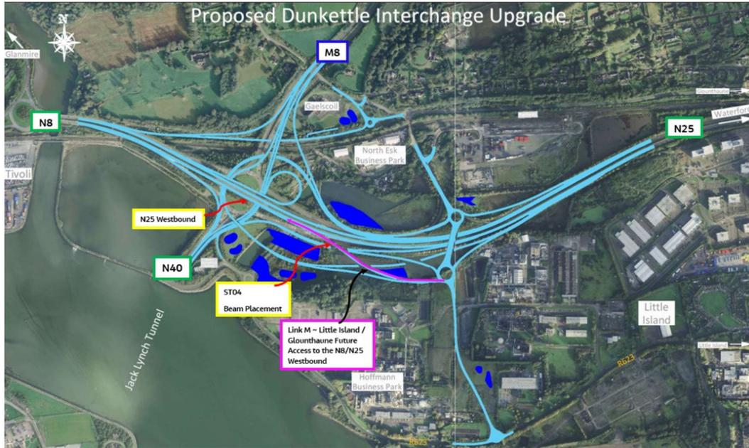
Layout Plan showing future Link M/N25 junction with Link M highlighted.
